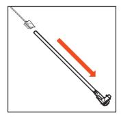
**Step 5**Push the cleaning rod through the inner barrel from front to back. Reverse this method to un-jam BBs.
