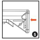
1 Make sure the selector switch is set to safe & fully retract the stock. 2 On both sides of the crane stock, push tabs together then pull to remove the buttpad. 3 Pull out tamiya battery connector from inside the stock. Slide the battery into stock side compartments. 4 Connect the battery to the connector. 5 Re-insert the battery cover, ensuring the tabs are locked in place.
